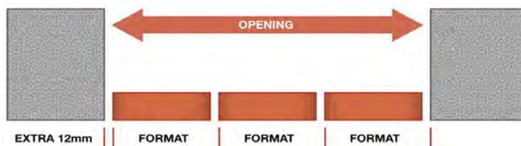
The height of brickwork measured conveniently between the tops of the courses is equal to the format height multiplied by the number of courses. The clear height of an opening (measured to the brickwork) is therefore greater by one joint than the coursing height of the opening - Figure 6.4
