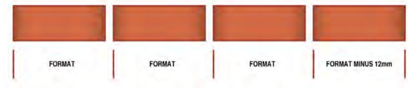
The actual widths of openings between brick reveals are greater by one 12mm joint than the width between format lines - Figure 6.3
