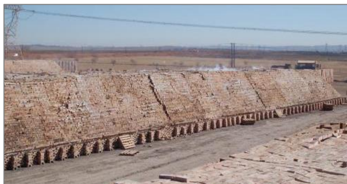
Figure 1: A full size clamp kiln. The model kilns takes a "slice" from the centre to duplicate firing conditions.
