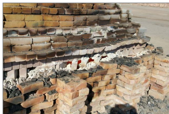
Figure 2: An open-air clamp kiln firing bricks
